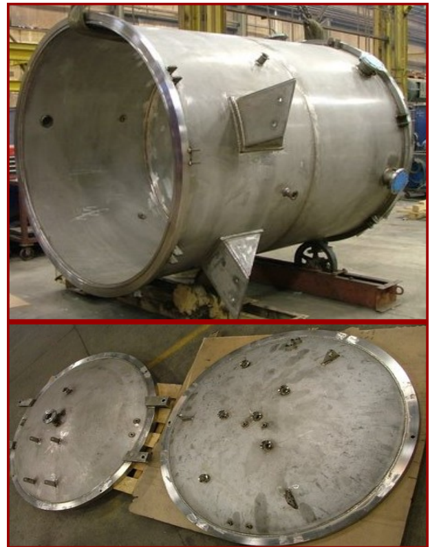
300 series SS 72" Dia. x 8' Long Flange faces machined parallel within +/- 0.01
