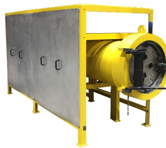
Test vessel 24" OD x 108" S/L 2000 PSIG @ 120 Deg F Quick Opening Closure
